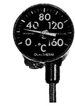
Dial hot spot winding temperature equipment including a current transformer may be specified. Energy from a current transformer added to the temperature of the top oil in the tank operate a bimetallic element to indicate the simulated hot spot temperature of one phase of the transformer winding. A pointer on the large weatherproof indicator dial gives visual indication, and switches are provided to actuate cooling equipment and to control alarm circuits.
