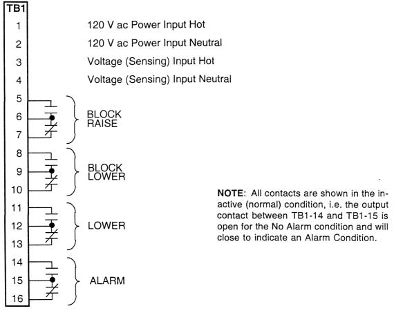
FIGURE 4 External Connections
