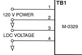
FIGURE 5 Power and Voltage Input Connections
