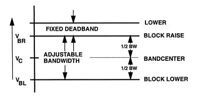
FIGURE 1 Setpoint Voltage Levels
