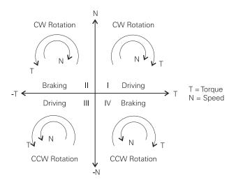
One method of dealing with negative torque and the current it produces is controlled deceleration. Voltage and frequency is reduced gradually until the motor is at stop. This would be similar to slowly removing your foot from the accelerator of a car. Many applications, however, require the motor to stop quicker, and the drive must be capable of handling the excess energy produced by motor when this is done.
