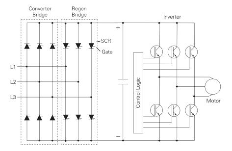
A simplified block diagram provides a clearer view of the regen process. When the motor needs motoring energy to accelerate or maintain speed against the inertia of a load, the converter bridge is turned on. When the motor is in the regenerative mode, it acts like a generator, supplying electrical energy back to the DC link. When the DC link voltage reaches a predetermined level the motoring SCRs are switched off and the regen (generating) SCRs are switched on.
