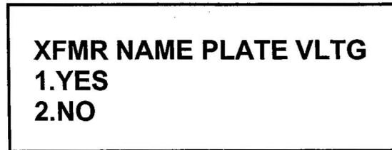
**Figure 14-4. Nameplate Voltage Selection Menu**
