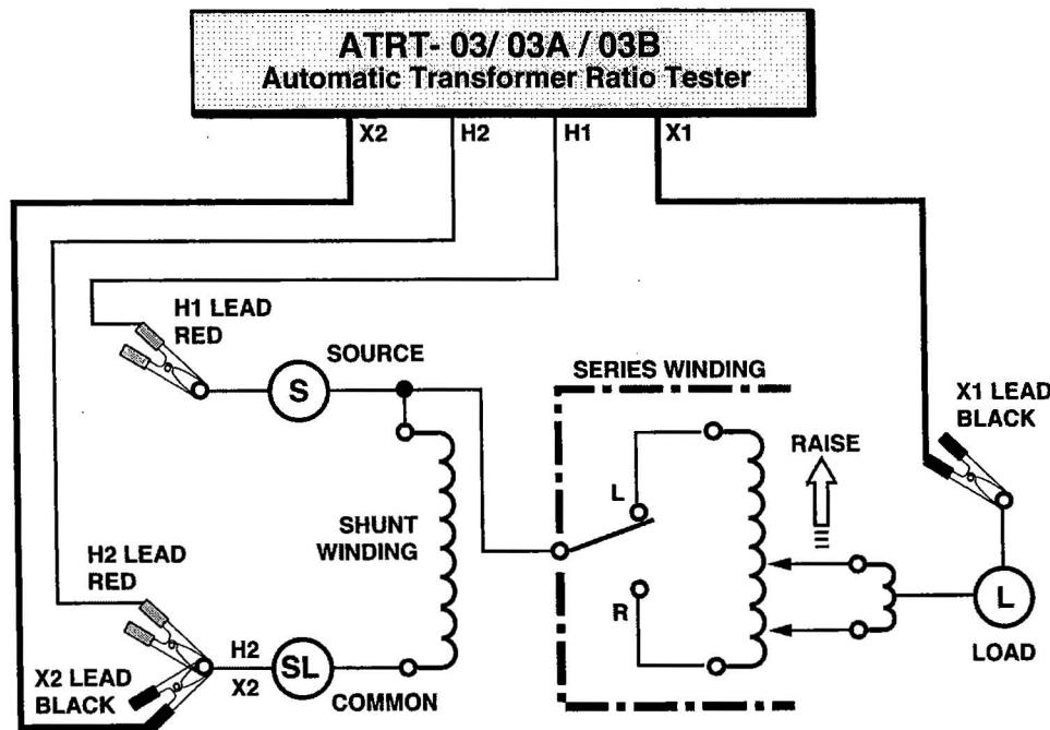
**Figure 13C. Typical Connection for Type A Voltage Regulator**
