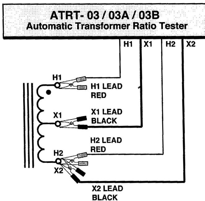
**Figure 13B. Typical Connection for Single-Phase Auto Transformer**
