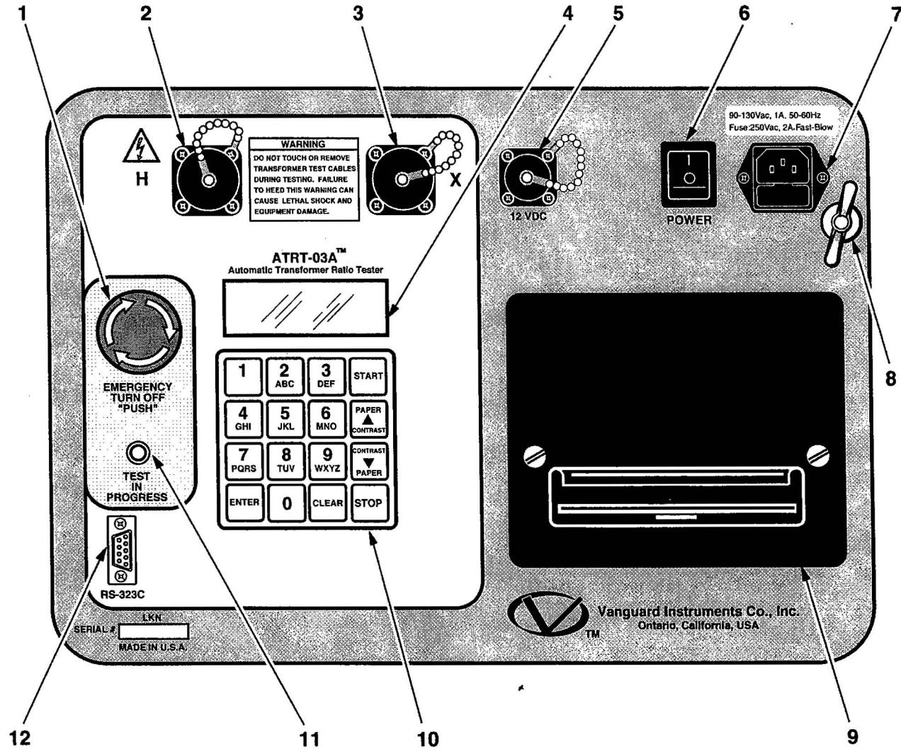
**Figure 7-2. Model ATRT-03A Front-Panel Controls, Indicators, and Connectors**
