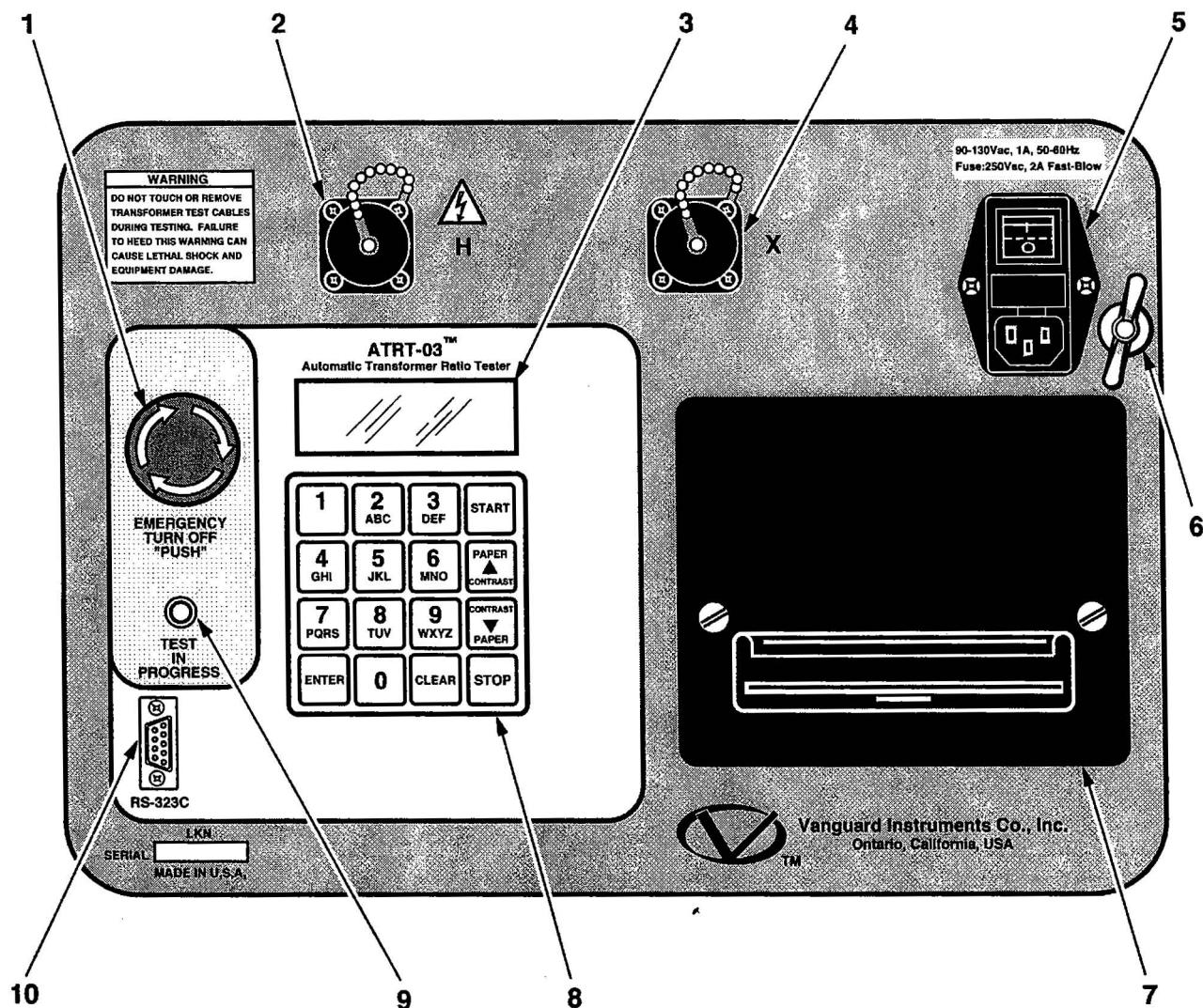
**Figure 7-1. Model ATRT-03 Front-Panel Controls, Indicators, and Connectors**
