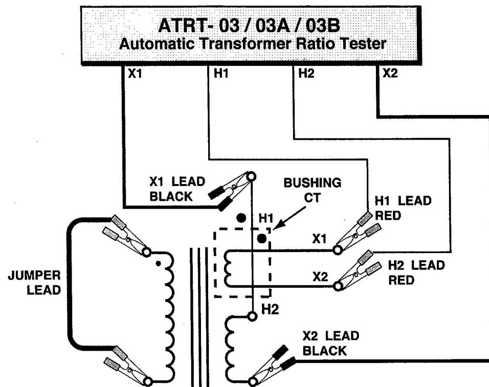
**Figure 13G. Typical Connection for Bushing-Mount-CT
