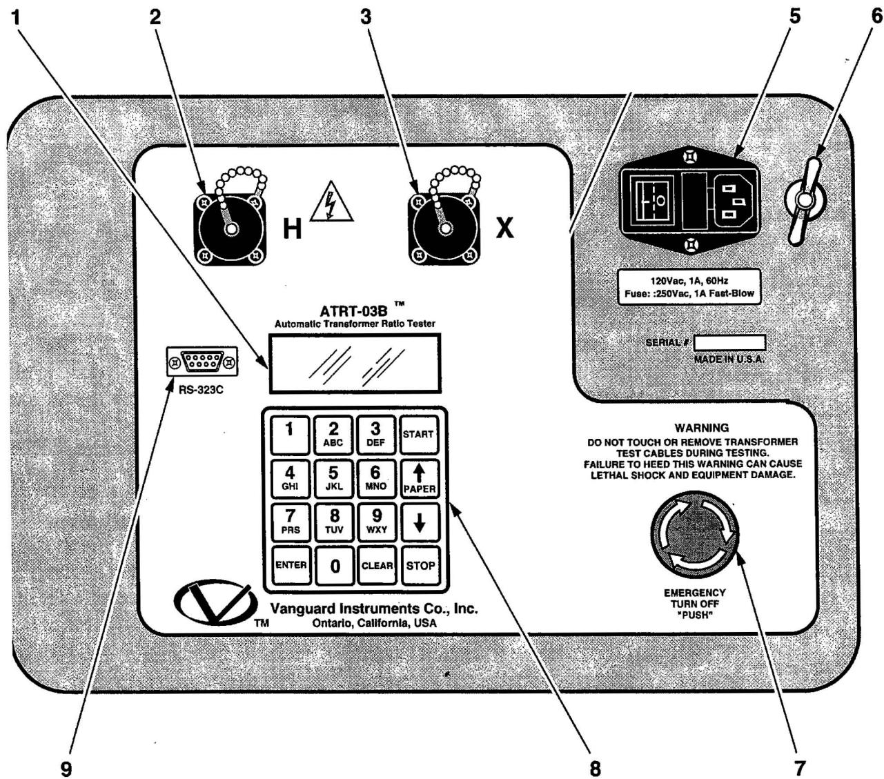
**Figure 7-3. Model ATRT-03B Front-Panel Controls, Indicators, and Connectors**
