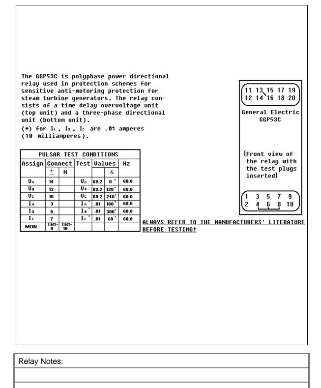
For Pick Up and Timing Test, assign current and voltage sources as indicated in the preset conditions table below.
