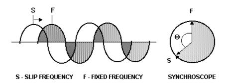
As "S" approaches "F", at some point (the advance angle) the relay will send a close signal, which will start the Timer. When "S" and "F" are in synchronous, the Timer will stop. The time indicated on the timer display is the advance time of the relay based on the preset slip frequency.
