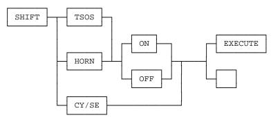
**HORN** Denotes the **HORN** key and indicates a start timer horn or a stop timer horn function. The **ON** and **OFF** keys from the **OUTPUTS**
