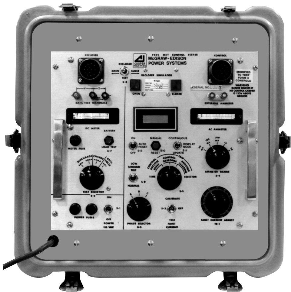
Figure 1. Type MET electronic recloser control tester.
