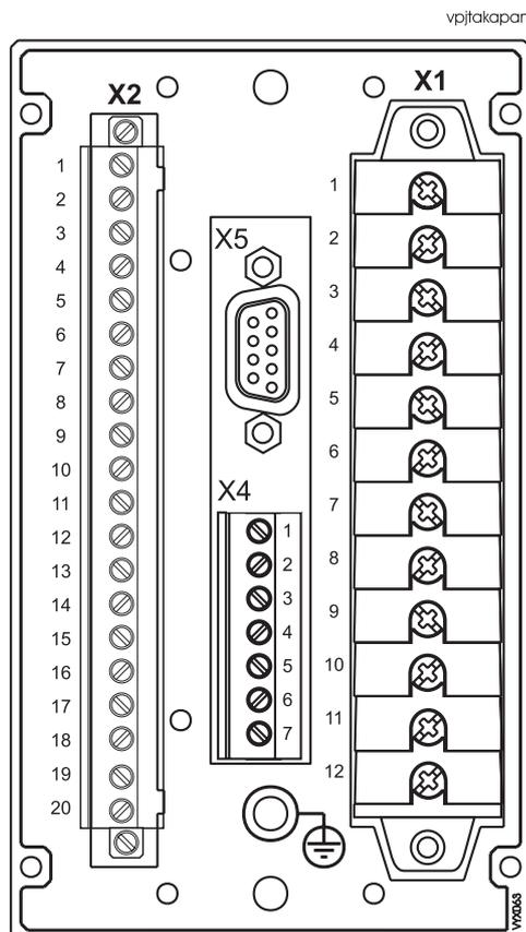
The VAMP 140 relay is connected to the protected object through the following measuring and control connections:
