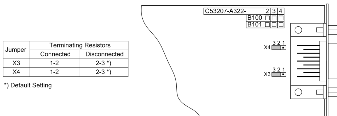
Figure 3-14 Position of the plug-in jumpers for the configuration of the terminating resistors at the interfaces PROFIBUS (FMS and DP), DNP3.0 and Modbus
