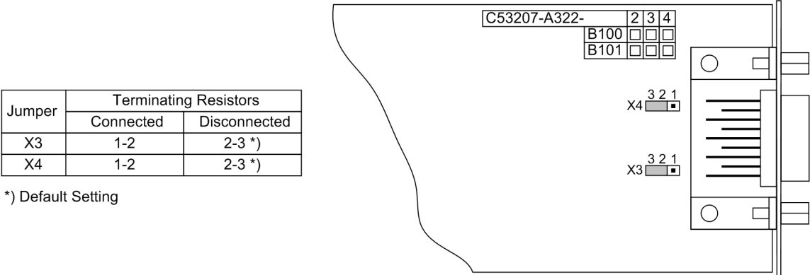
Figure 3-24 Position of the plug-in jumpers for the configuration of the terminating resistors at the Profibus (FMS and DP), DNP 3.0 and Modbus interfaces.
