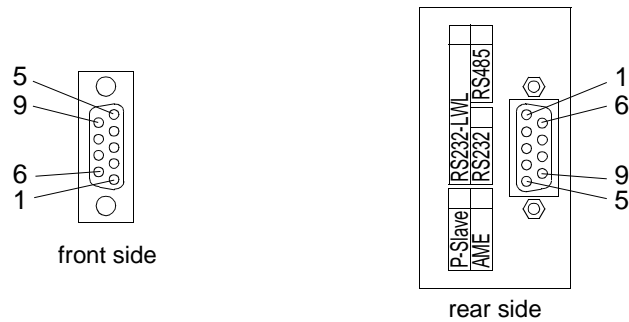
Figure 2-13 9 pin D-subminiature Connector
