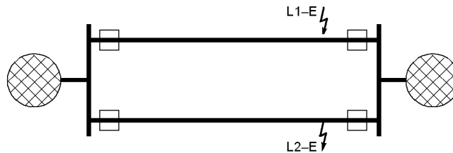
Figure 2-5 Multiple fault on a double-circuit line
