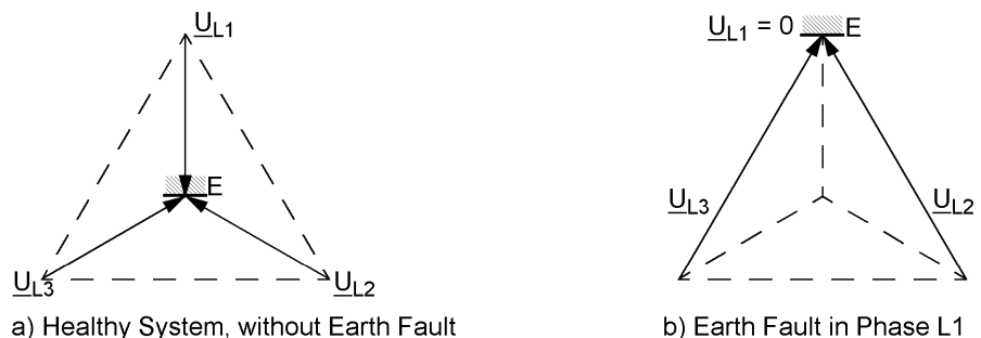
Figure 2-102 Earth fault in non-earthed neutral network
