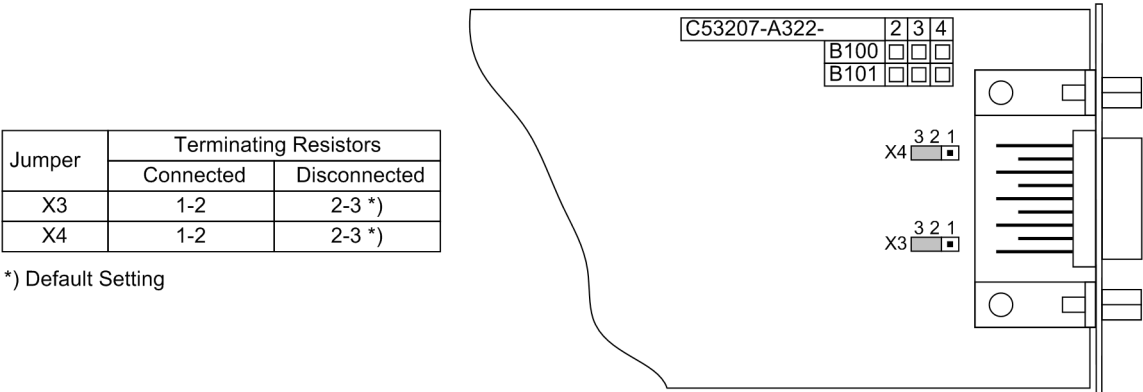
Figure 3-14 Location of the jumpers for configuring the PROFIBUS and DNP 3.0 interface terminating resistors
