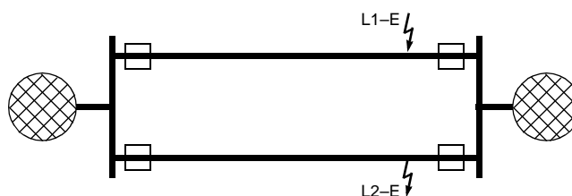
Figure 6-13 Multiple fault on a double-circuit line
