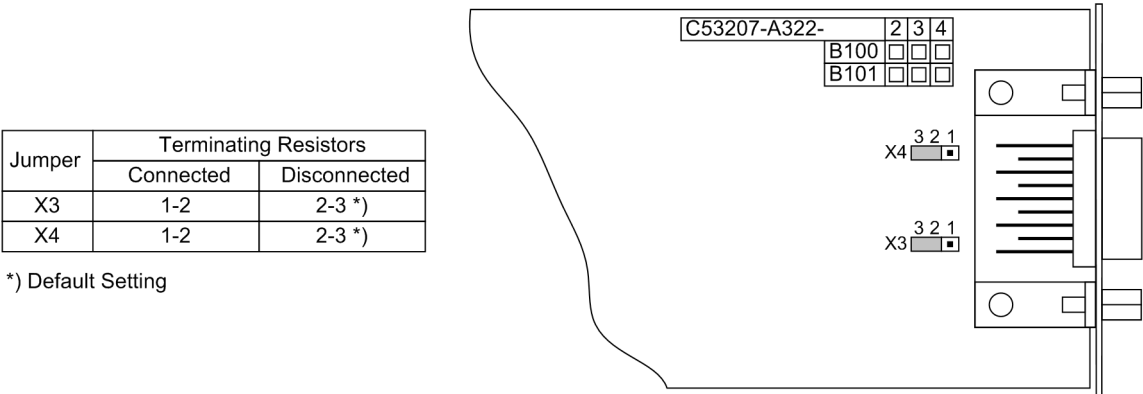
Figure 3-11 Position of the plug-in jumpers for the configuration of the terminating resistors at the interfaces Profibus (FMS and DP) and DNP 3.0 interface.
