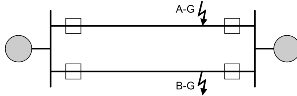
Figure 2-5 Multiple fault on a double-circuit line
