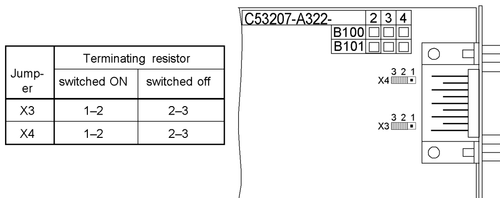
Figure 3-7 Position of the jumpers for configuration of termination resistors of the PROFIBUS FMS and PROFIBUS DP interface
