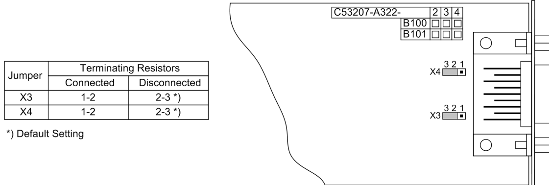
Figure 3-10 Position of the plug-in jumpers for the configuration of the terminating resistors at the Profibus (FMS and DP), DNP 3.0 and Modbus interfaces.
