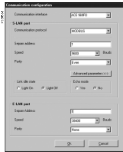
SFT2841: communication configuration window for ACE969FO.
