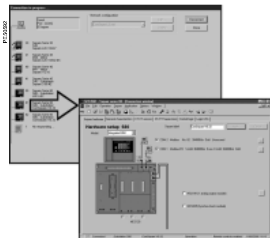
Access to parameters and settings for a Sepam series 80 connected to a communication network.
