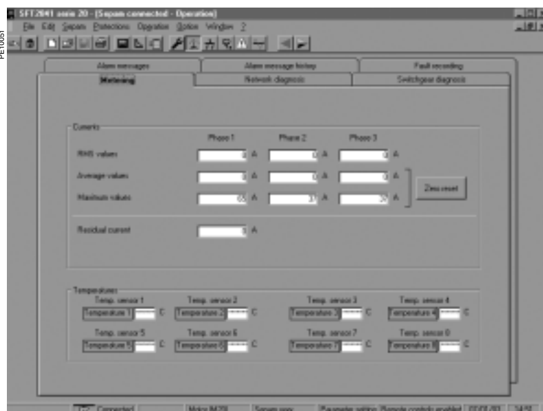
Example of a measurement display screen (Sepam M20).
