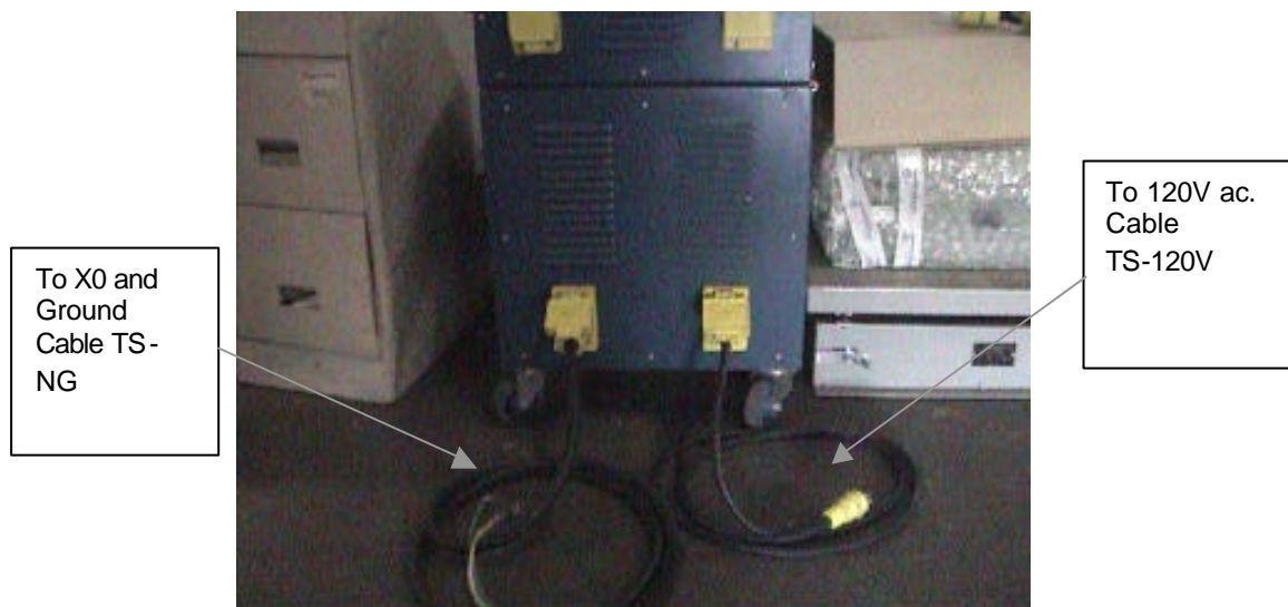
Figure 1. Connections for direct connection to system star-point
