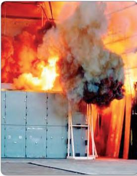
While solidly grounded systems are an improvement over ungrounded systems, and speed the location of faults, they lack the current limiting ability of resistance grounding and the extra protection this provides. The destructive nature of arcing ground faults in solidly grounded systems is well known and documented and are caused by the energy dissipated in the fault.
