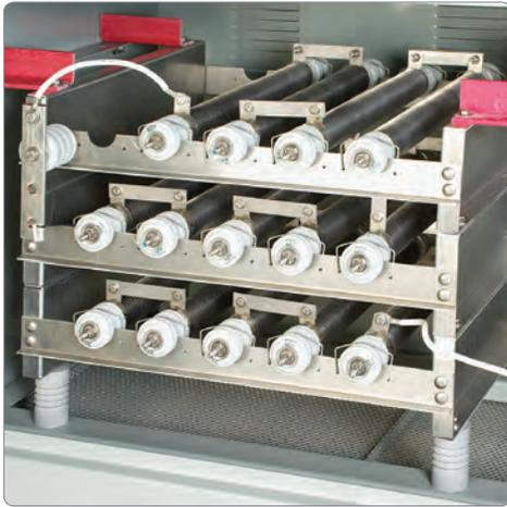
All I-Gard's low resistance grounding products are standardized on the edgewound element design. Because of the rapid heating and very high temperatures encountered, this design has been proven superior for the NGR application.
