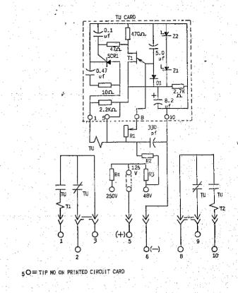
Fig. 1-Internal Connection For Relay Type SAM 11D21 and up Front View (208A2423)
