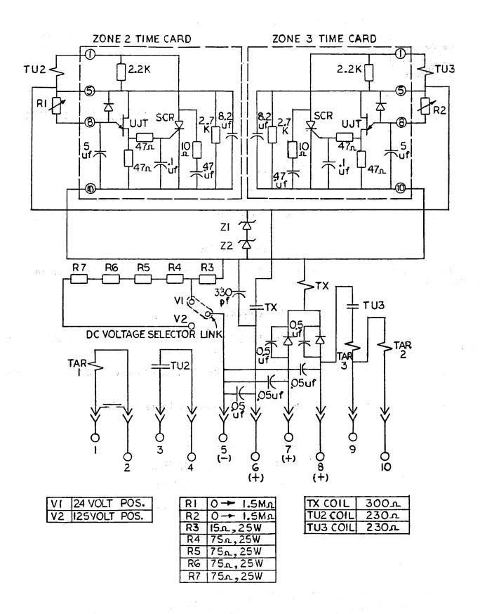
Fig. 1 (0285A5622-0) Internal Connections for SAM99AF Relay
