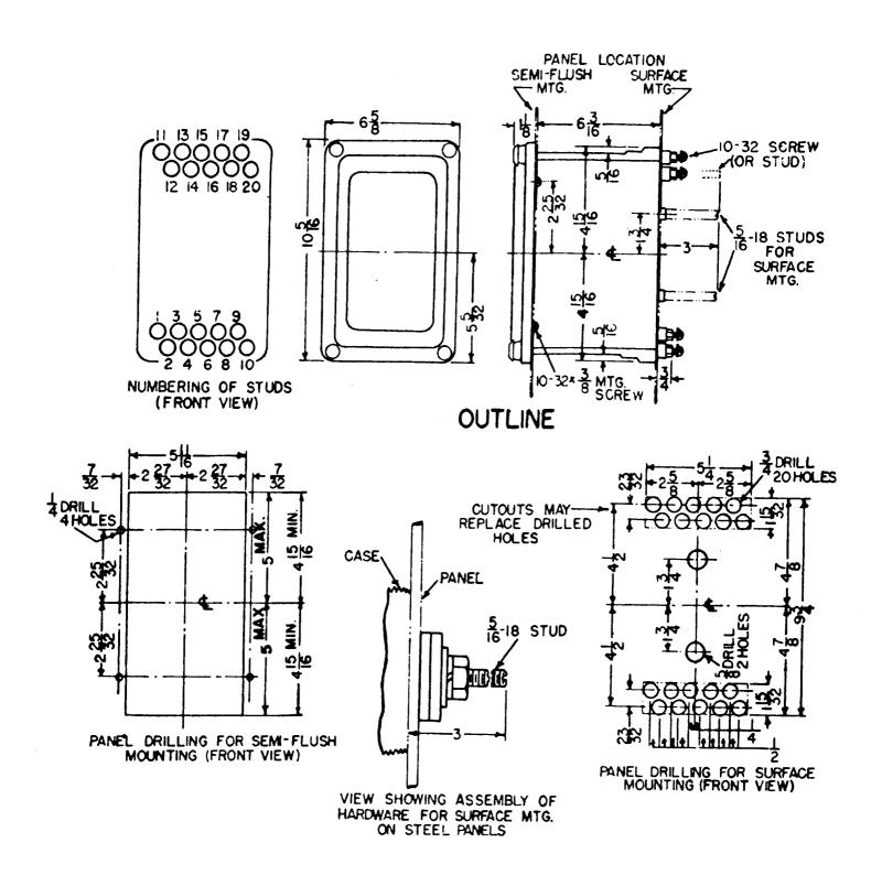
FIG. 2 (K-6209272-2) Outline And Panel Drilling Dimensions For Model 0208A8459 Relay
