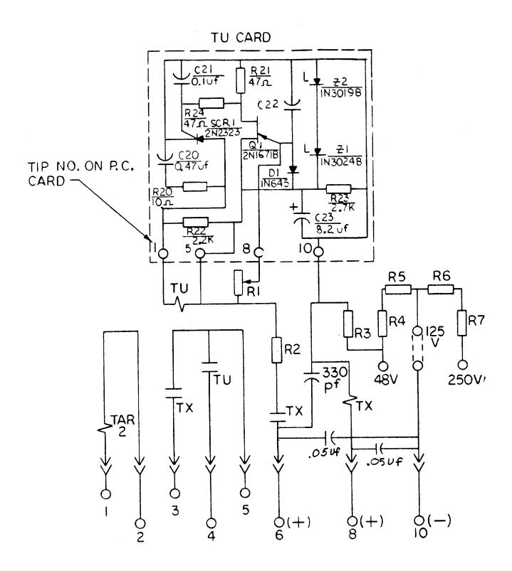
FIG. 1 (0246A2409[3]) Internal Connections For 12SAM17G(-)A
