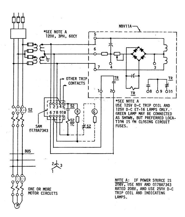
FIG. 2 (0246A6817-0) External Connection Diagram For 0178A7343 SAM Relay
