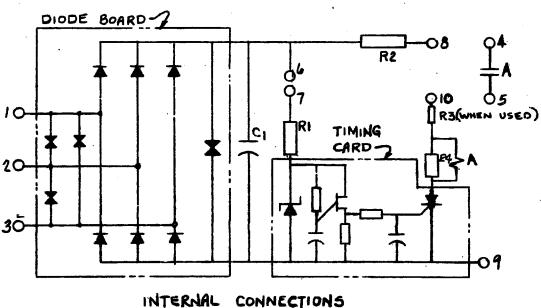
FIG. 1 (0178A9089-3) Outline And Internal Connections For 0178A734C SAM Relay
