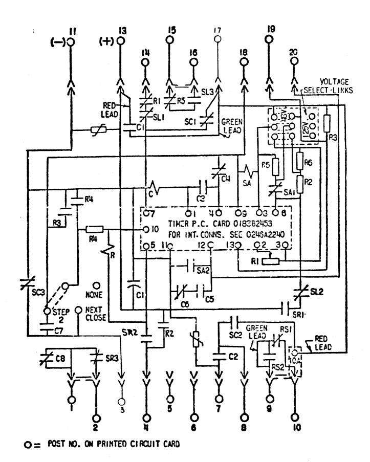
Figure 1 (0269A3033-0) Internal Connections Diagram for the 12NLR99AD001A Relay
