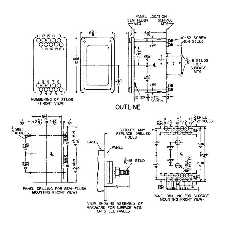
FIG. 2 (K-6209272-2) Outline And Panel Drilling - NAA27AB Relay
