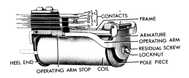
FIG. 4 (8012106) Typical Telephone Relay Unit Showing Nomenclature
