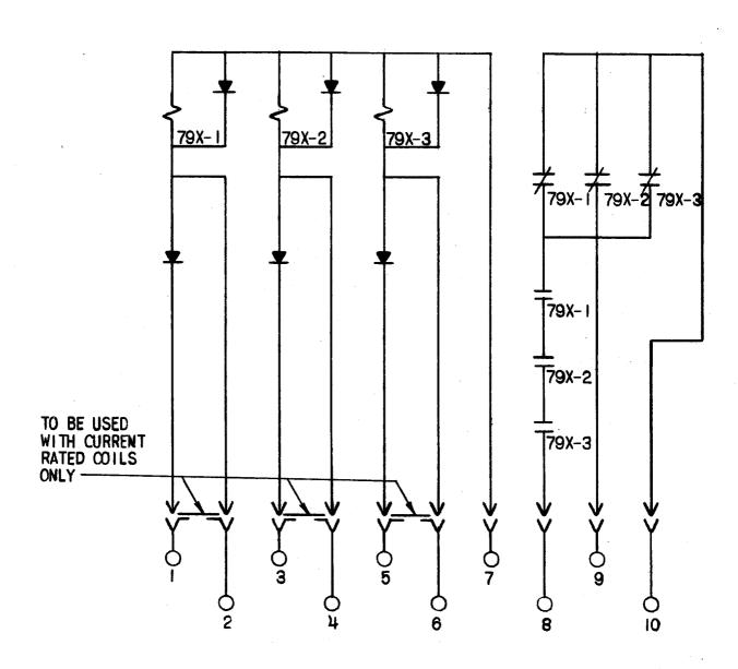
FIG. 1 (0246A3664) Internal Connections For 0208A8419
