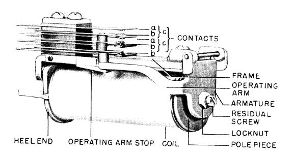
FIG. 3 (8012106) Typical Telephone Relay Unit Used In NAA Relays
