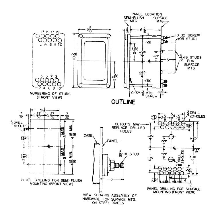
FIG. 2 (K-6209272-2) Outline And Panel Drilling Dimensions For NAA27Y(-)A
