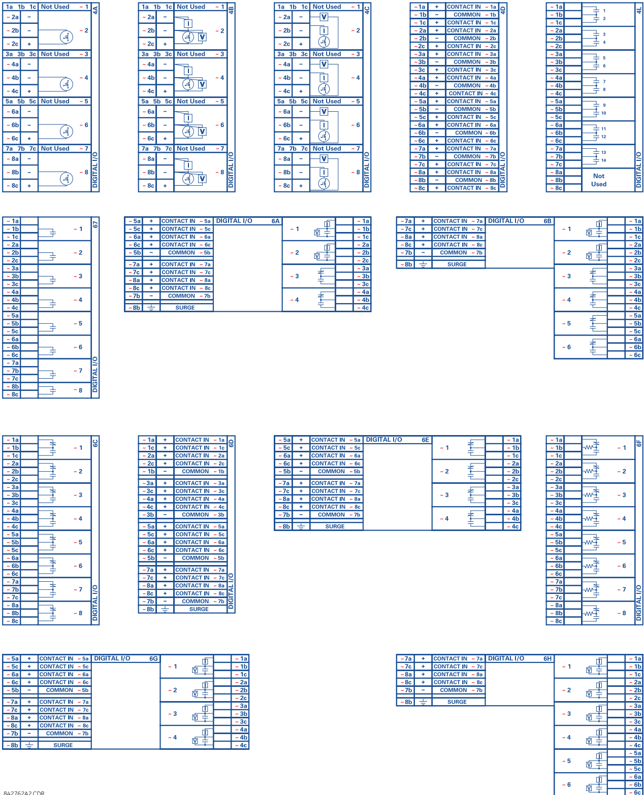
Figure 3-17: DIGITAL INPUT/OUTPUT MODULE WIRING (1 of 2)
