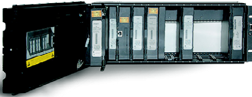
Figure 3-7: UR MODULE WITHDRAWAL AND INSERTION (ENHANCED FACEPLATE)
