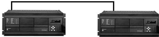
Figure 3-27: BACK TO BACK CONNECTION
