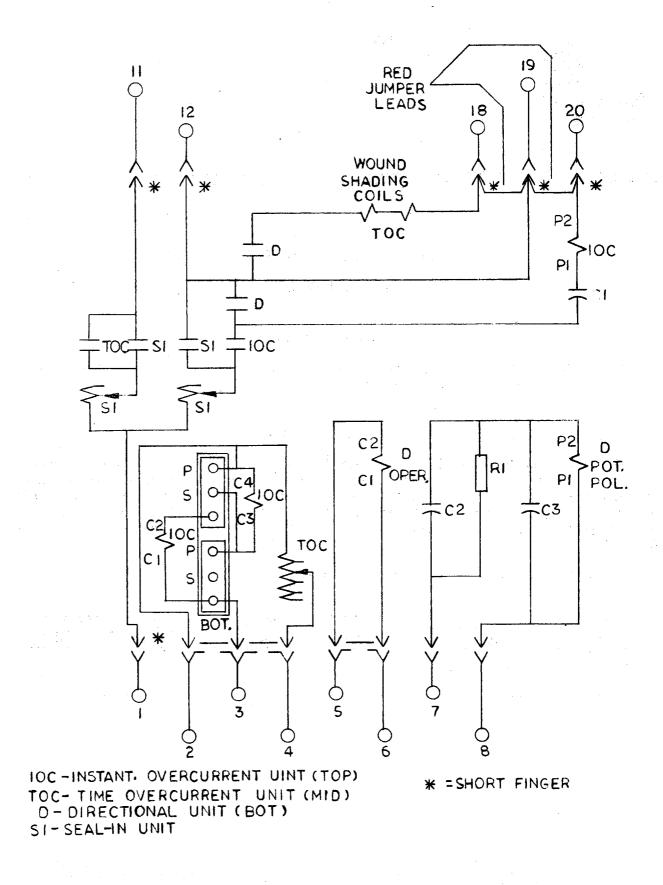
Fig. 1 (0257A6174-0) Internal Connections for JBC99AB(-)A Relays (Front View)
