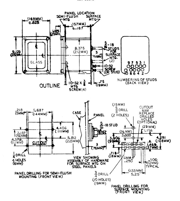
Fig. 4 (6209271-5) Outline and Panel Drilling for Drawout Relays - Size S1
