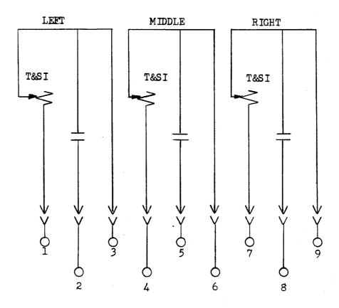
Fig. 2 (0178A9168-0) Internal Connections of the HAA99AE Relay (Front View)
