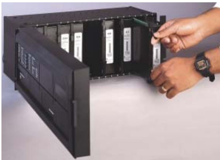
Figure 3-5: UR MODULE WITHDRAWAL/INSERTION
