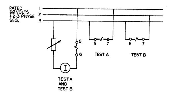
Fig. 5 (0275A3258-0) Testing Connections for Type CFW11E Relay Using Three Phase Voltage Source
