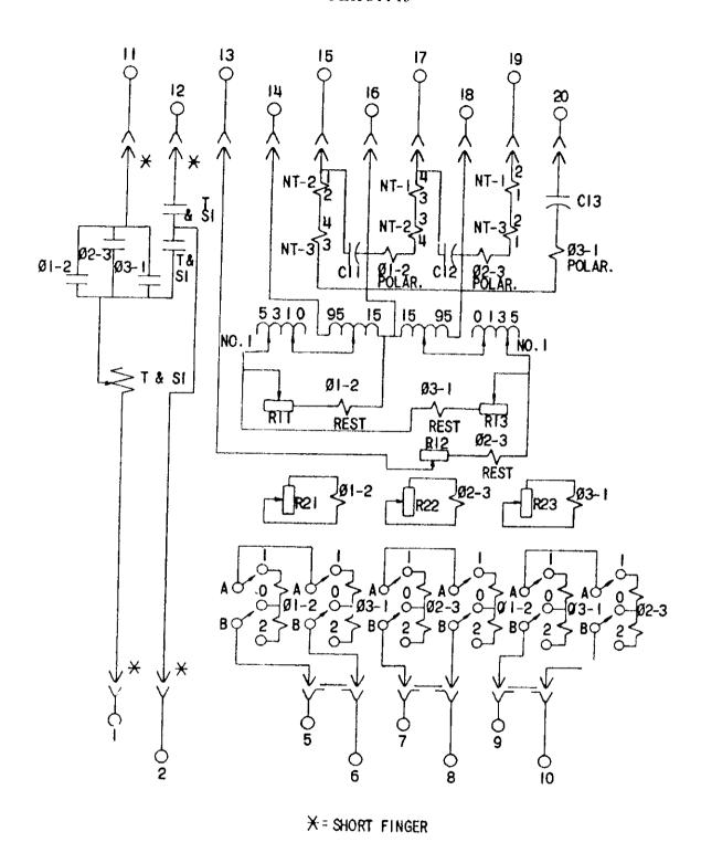
FIG. 1 (0227A7023-0) Internal Connections Diagram for the CEY56A Relay (Front View)
