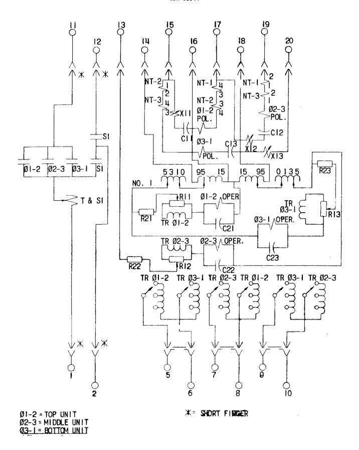
FIG. I (022/A7013-0) Internal Connections Diagram For The CEY51B Relay (Front View)
