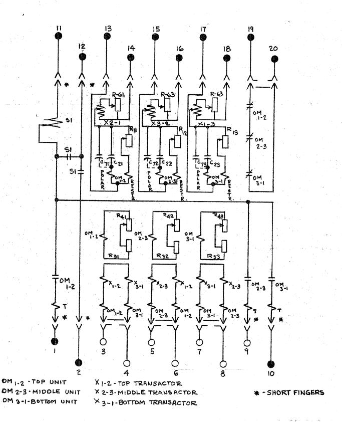
FIG. 1 (0165A6054-1) SH. 1 INTERNAL CONNECTIONS DIAGRAM FOR THE CEB13J RELAY (FRONT VIEW)
