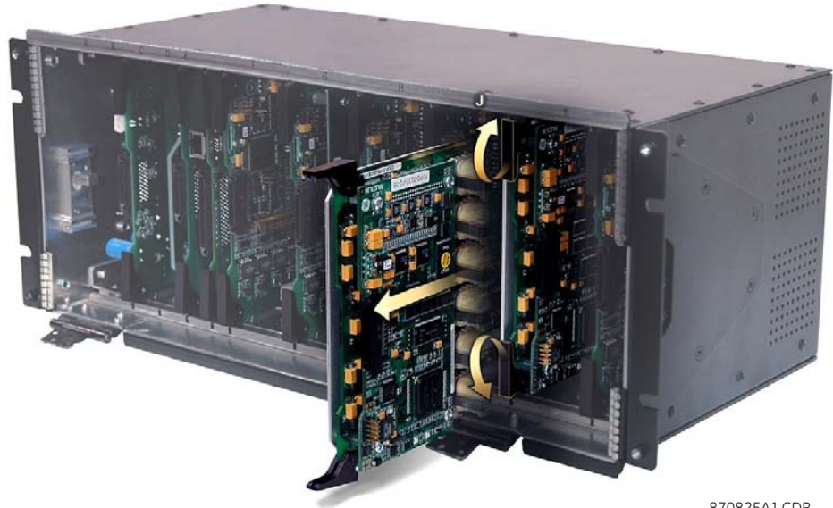
Figure 16: Module withdrawal and insertion
