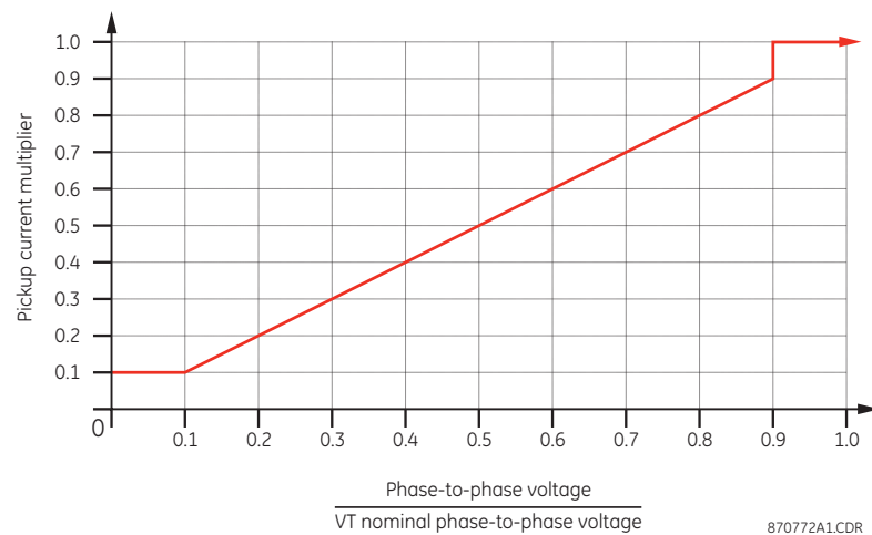
Figure 93: Phase time overcurrent voltage restraint characteristic
