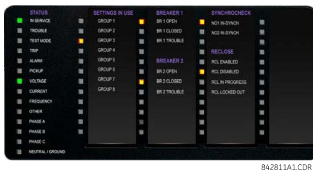
Figure 4-18: TYPICAL LED INDICATOR PANEL FOR ENHANCED FACEPLATE
