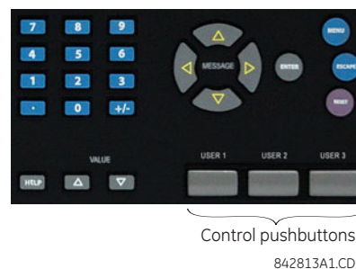
Figure 5-5: CONTROL PUSHBUTTONS (ENHANCED FACEPLATE)
