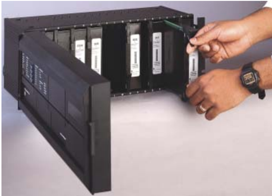
Figure 3-5: UR MODULE WITHDRAWAL/INSERTION
