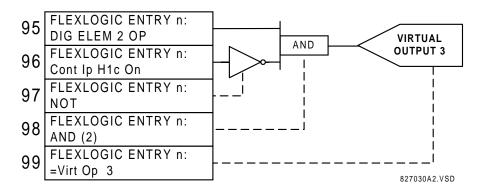
Figure 5–7: FLEXLOGIC™ EQUATION & LOGIC FOR VIRTUAL OUTPUT 3
