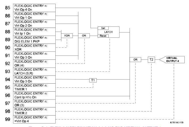
Figure 5-8: FLEXLOGIC™ EQUATION & LOGIC FOR VIRTUAL OUTPUT 4
