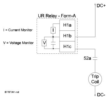
Figure 5-10: TRIP CIRCUIT - EXAMPLE 1
