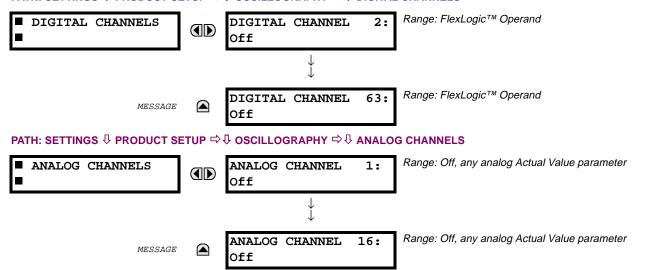
Oscillography records contain waveforms captured at the sampling rate as well as other relay data at the point of trigger. Oscillography records are triggered by a programmable FlexLogic<sup>™</sup> operand. Multiple oscillography records may be captured simultaneously.
