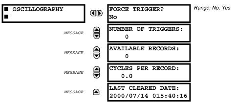
This menu allows the user to view the number of triggers involved and number of oscillography traces available. The 'cycles per record' value is calculated to account for the fixed amount of data storage for oscillography. See also the SETTINGS \ PRODUCT SETUP \ OSCILLOGRAPHY section.
