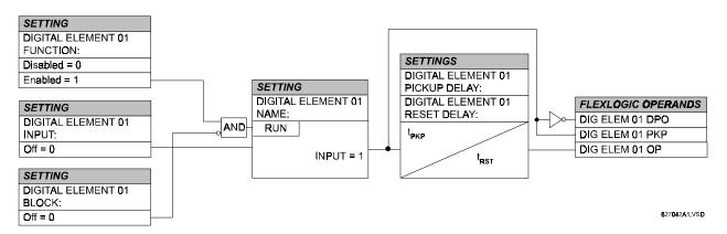
Figure 5–9: DIGITAL ELEMENT SCHEME LOGIC
