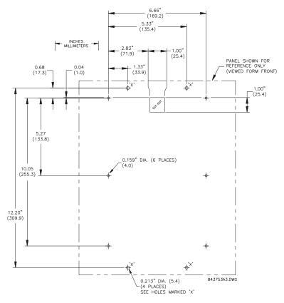
Figure 3-3: UR VERTICAL SIDE MOUNTING REAR DIMENSIONS
