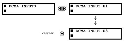
Hardware and software is provided to receive signals from external transducers and convert these signals into a digital format for use as required. The relay will accept inputs in the range of –1 to +20 mA DC, suitable for use with most common transducer output ranges; all inputs are assumed to be linear over the complete range. Specific hardware details are contained in the HARDWARE chapter.
