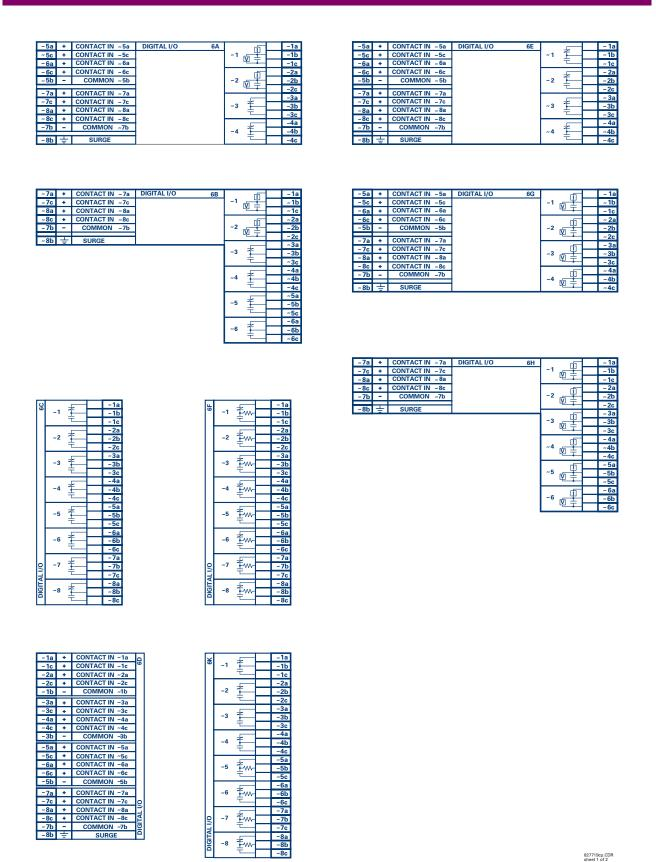
Figure 3-11: DIGITAL I/O MODULE WIRING (Sheet 1 of 2)
