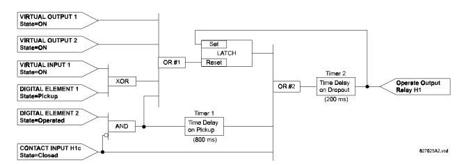
Figure 5-2: EXAMPLE LOGIC SCHEME
