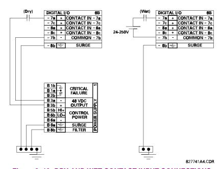
Figure 3–13: DRY AND WET CONTACT INPUT CONNECTIONS
