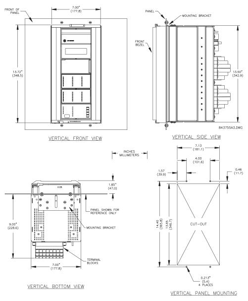
Figure 3-1: UR VERTICAL MOUNTING AND DIMENSIONS
