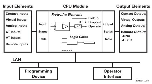
Figure 1-2: UR CONCEPT BLOCK DIAGRAM
