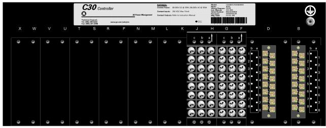
Figure 3-6: REAR TERMINAL VIEW
