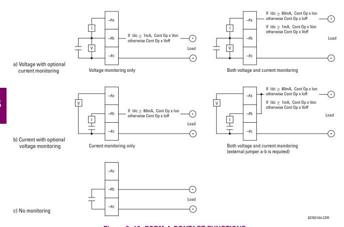
Figure 3-10: FORM-A CONTACT FUNCTIONS
