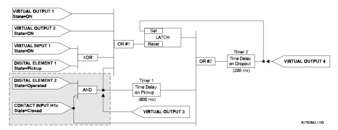
Figure 5–3: LOGIC EXAMPLE WITH VIRTUAL OUTPUTS
