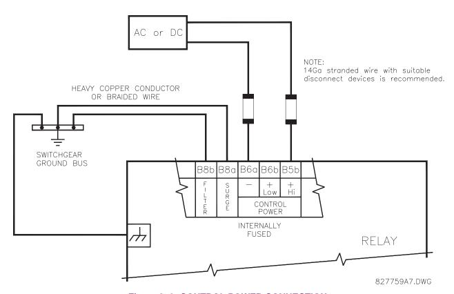
Figure 3-9: CONTROL POWER CONNECTION
