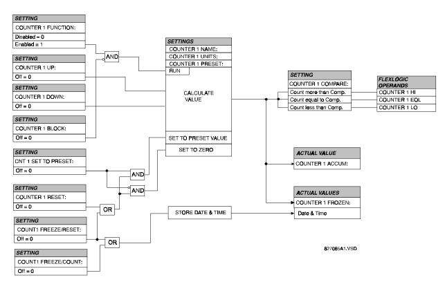
Figure 5–12: DIGITAL COUNTER SCHEME LOGIC
