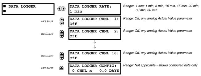
The data logger is used to sample and record up to sixteen analog parameters at a sampling rate that is defined by the user. This recorded data may be downloaded to the URPC software where it is displayed with 'parameters' on the vertical axis and 'time' on the horizontal axis. All data is stored in non-volatile memory which means that the information is retained when power to the relay is lost.
