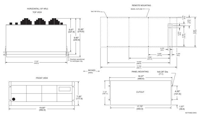
Figure 3-4: UR HORIZONTAL MOUNTING AND DIMENSIONS
