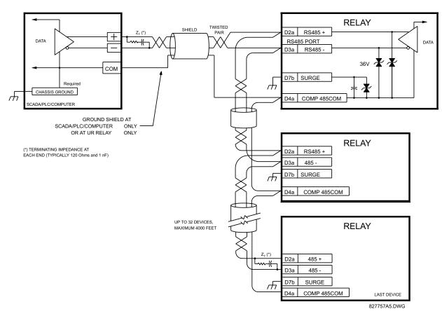
Figure 3–17: RS485 SERIAL CONNECTION
