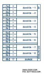
Figure 3-14: TRANSDUCER I/O MODULE WIRING
