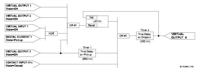
Figure 5-5: LOGIC FOR VIRTUAL OUTPUT 4
