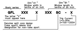
Example: To order a rectangular sensor with a 4.1 x 7.1 window and a 5-60A trip current, the catalog number would be GFL 041 X 071-1.
