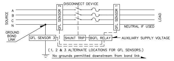
To determine if the neutral is grounded in only one place at the service entrance (in accordance with The National Electrical Code);
