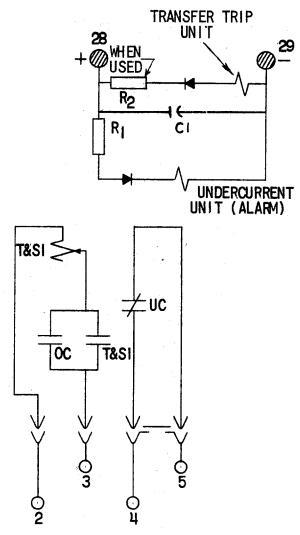
HIGH VOLTAGE STUDS (28 & 29) PROJECT THRU REAR OF CASE. LEADS & BUSHINGS MUST BE REMOVED FROM STUDS 28 & 29 BEFORE CRADLE CAN BE WITHDRAWN.
