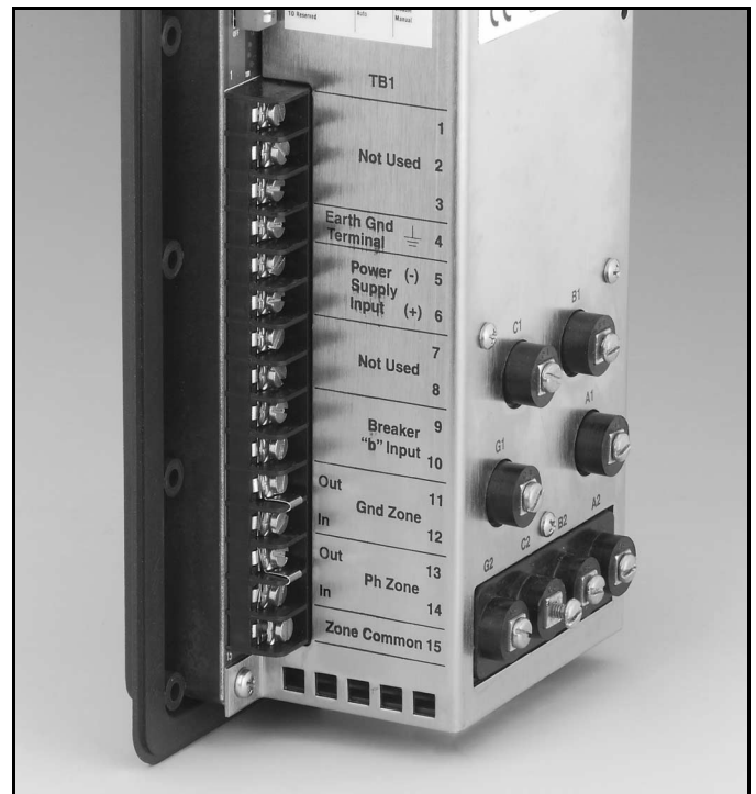
Fig. 1-5 Installed Jumpers in Place on Terminal Block TB-1 Disabling the Zone Interlocking Feature
