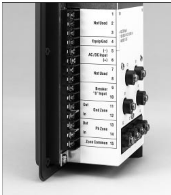
Figure 1-6 Installed Jumpers in Place on Terminal Block TB-1 Disabling the Zone Interlocking Feature
