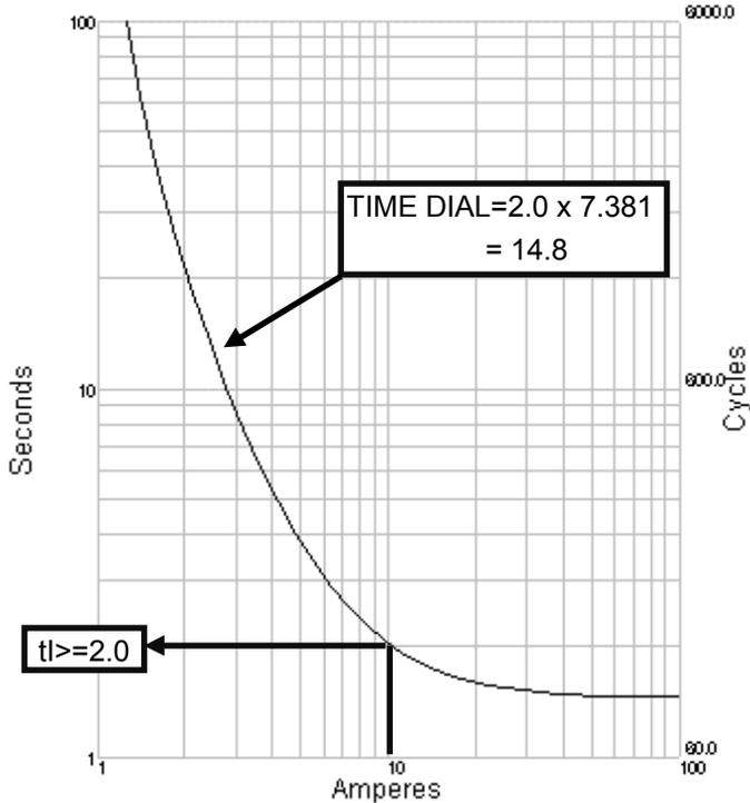
Figure 9: Example of IEEE Very Inverse Curve Time Delay Setting Determination
