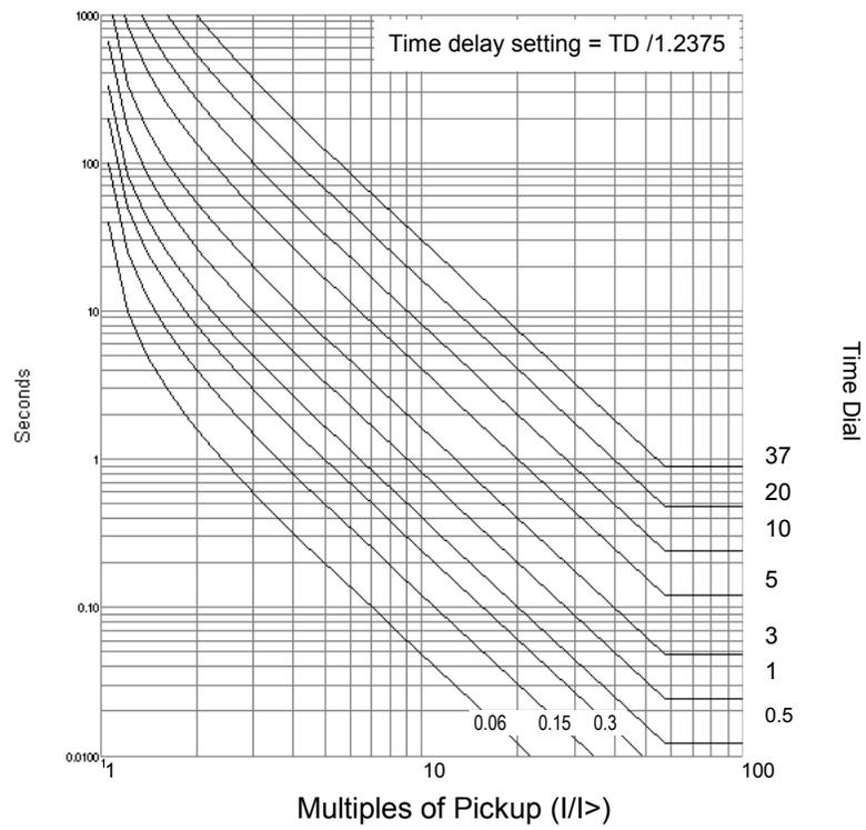
**Figure 14 - IEC Extremely Inverse (c) Curve**
