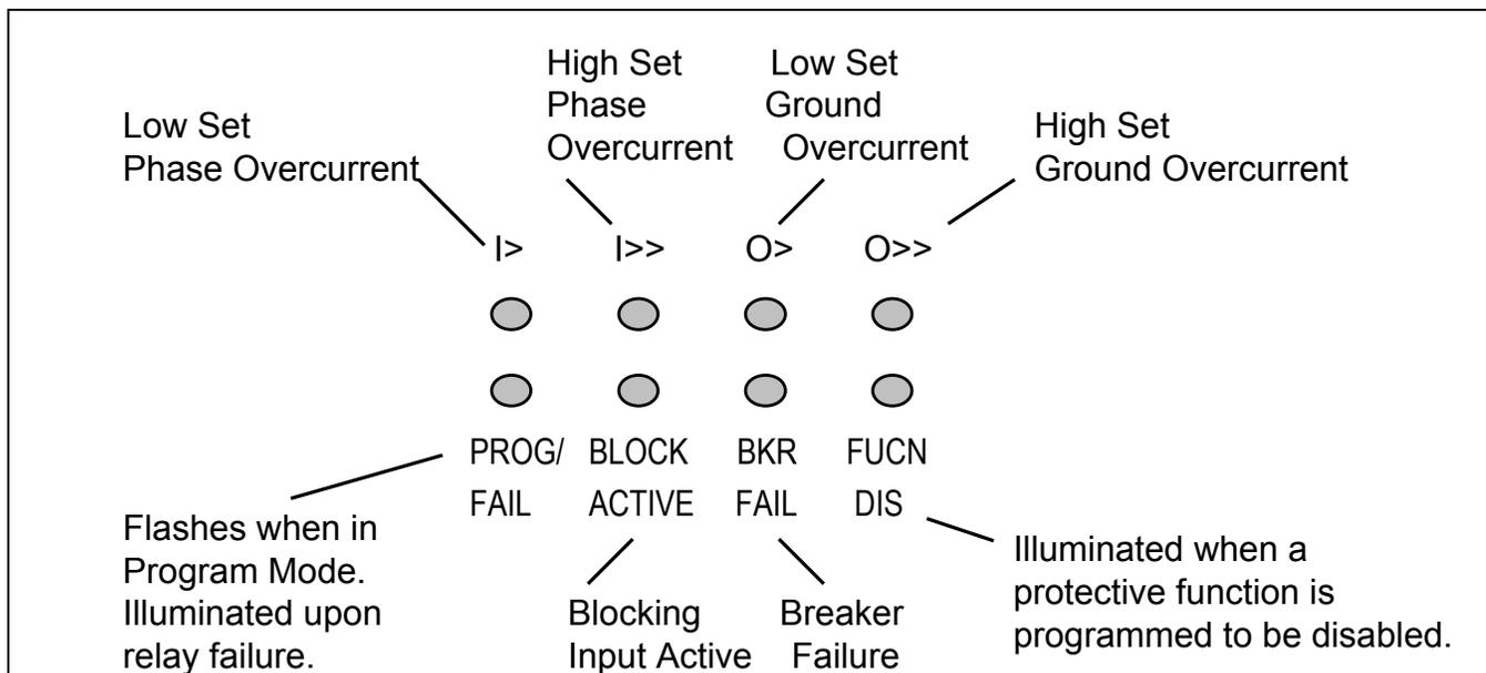
FIGURE 5: Front Panel Targets on IM30AE Relay
