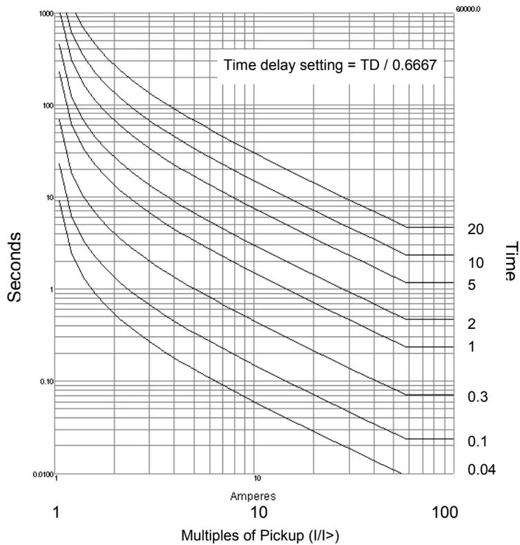
Figure 13 - IEC Very Inverse (B) Curve
