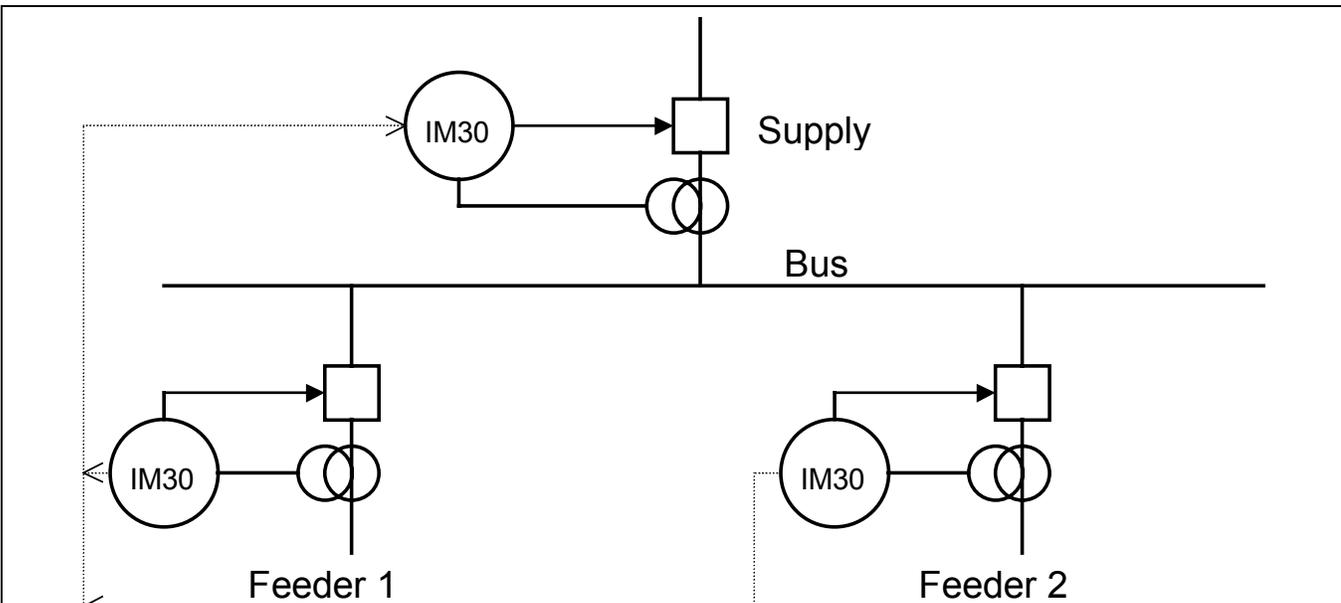
FIGURE 20: Typical Implementation of the IM30AE's Fast Bus Trip Logic
