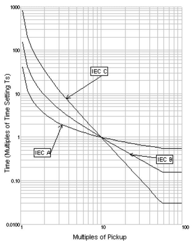
Figure 11: Easy Set Curves for IEC Curve Set
