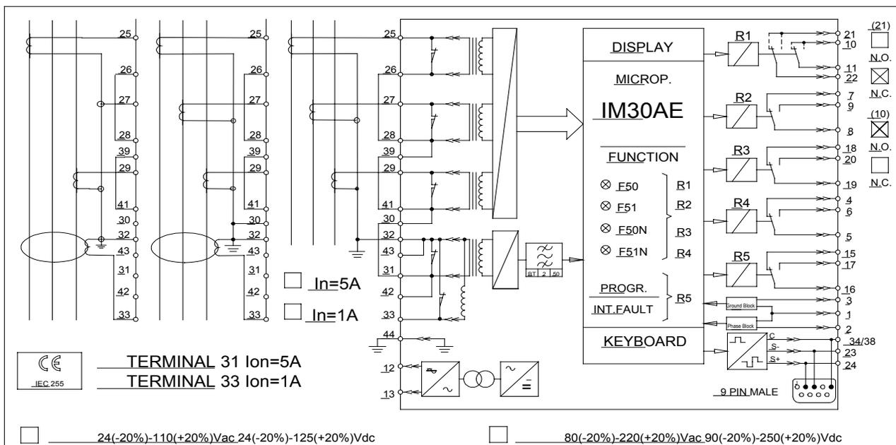
FIGURE 4 - Wiring Diagram for the IM30AE
