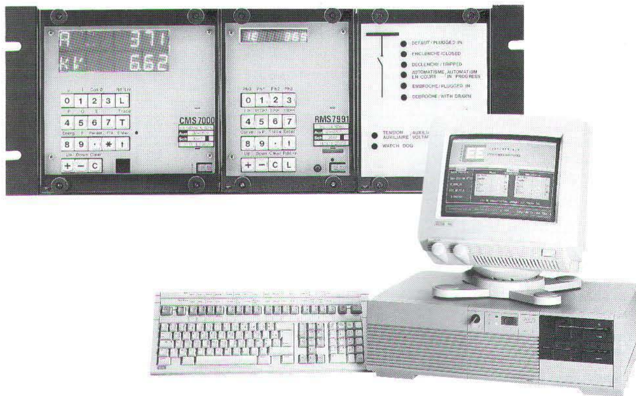
Set of 3 PROCOM cases mounted in 19" RACK with microcomputer connection.
