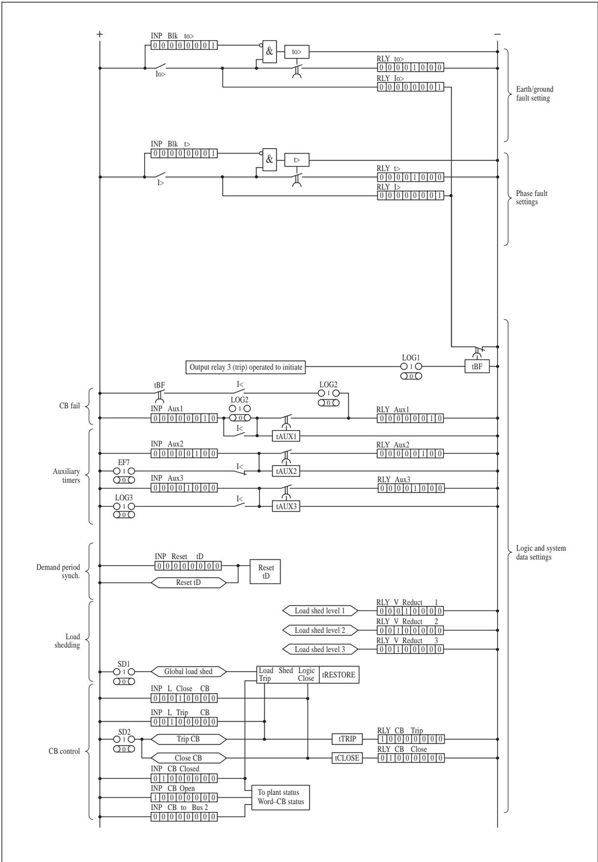
Figure 18. Scheme logic diagram: Midos measurement centre Type KMPC 130
