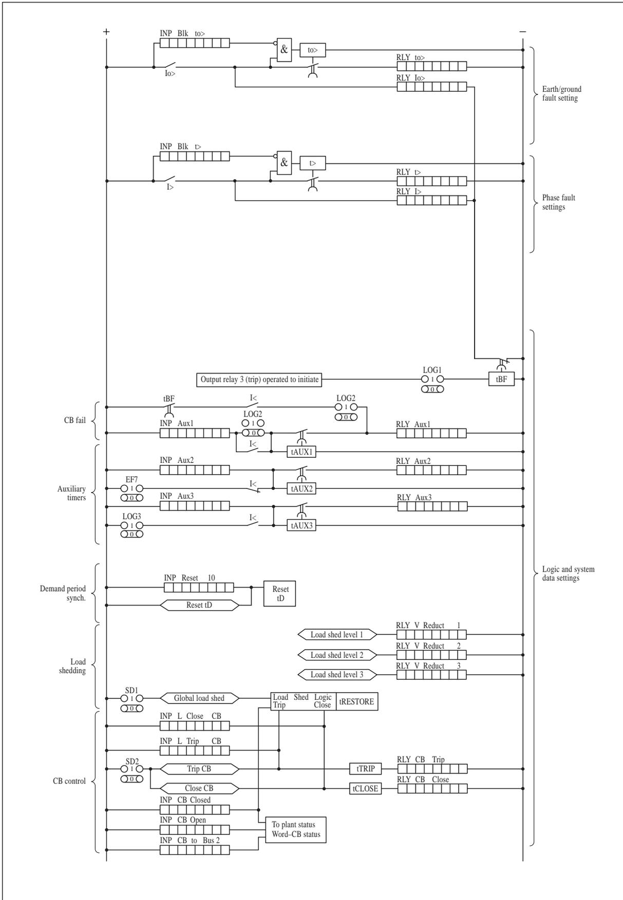
Figure 17. Scheme logic diagram: Midos measurement centre Type KMPC 130
