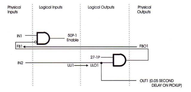
In the above example, the 50-1 function is enabled when IN1 is HIGH (denoted by a C in the Programmable Input map) AND FB1 is LOW (denoted by an O in the Programmable Input map).
