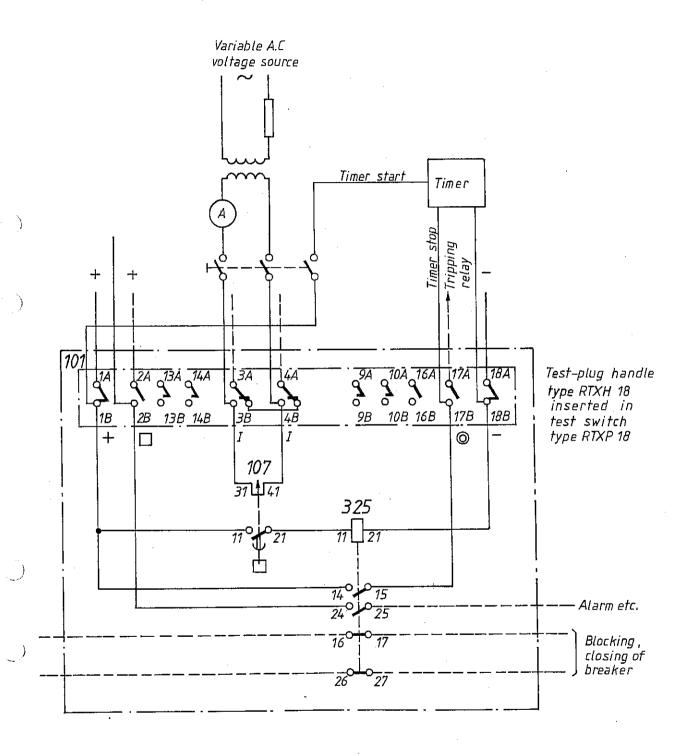
Fig. 1 Secondary injection test of RVAB
